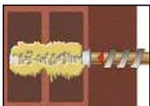
7. Push the threaded rod into the anchor hole while turning slightly to ensure positive distribution of the adhesive until the embedment depth is reached. The anchor should be free of dirt, grease, oil or other foreign material.
