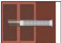
5. Insert the sleeve into the bore hole.
