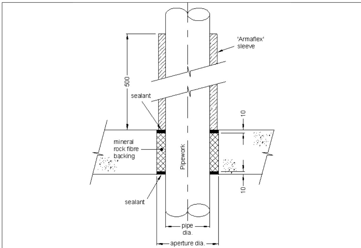
**A.3.1.1 Pipes with local interrupted (minimum 500 mm) or continuous interrupted 25 mm thick Armacell 'Class O Armaflex' Insulation**
