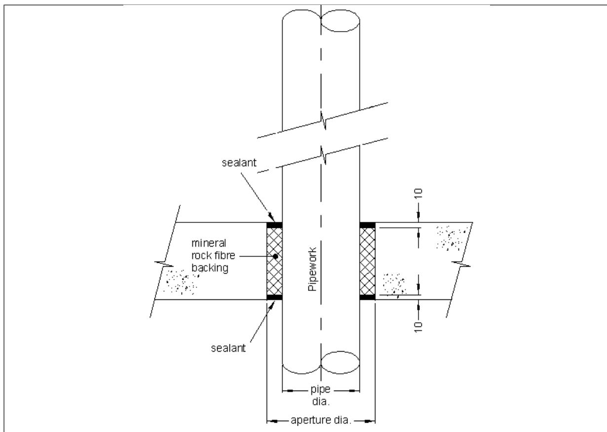
**A.3.2.1 Pipes without insulation**
